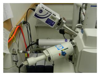
In picture to left, locate/label: A) EBSD Detector B) EDS Detector C) CL Detector D) Secondary (SE) Detector
